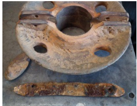
Bronze diaphragm casting and cross peg
