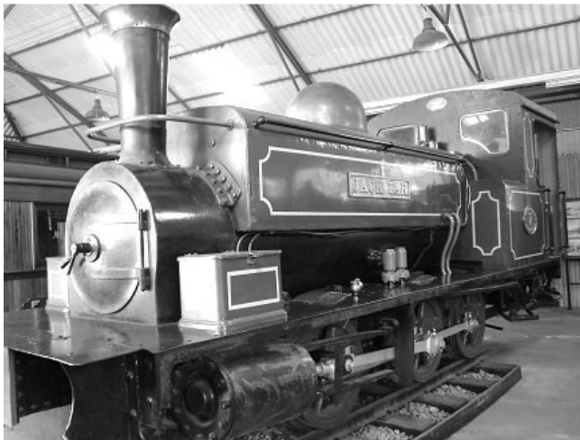
Manning Wardle 0-6-0, similar to one of the locomotives as used on the Tregantle Military Railway.
