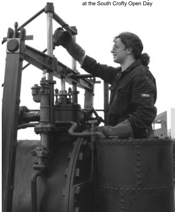
Tom Rowan oils the crosshead guides at the South Crofty Open Day
