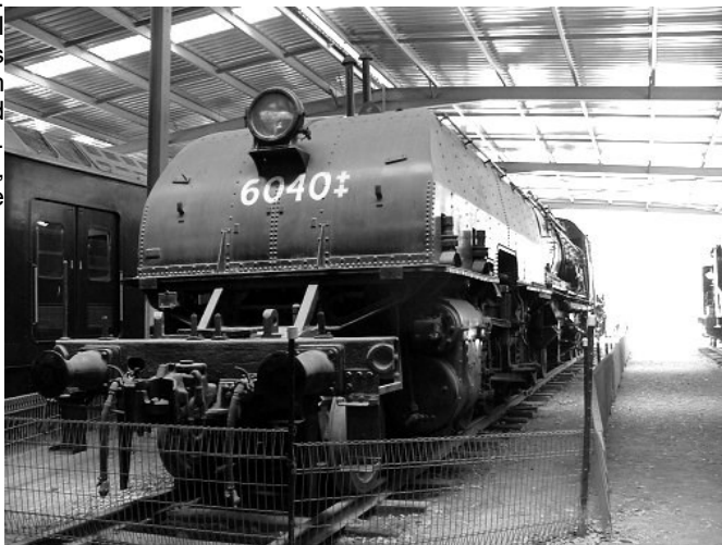
Garratt-type locomotive with two engines, each with eight wheels fed by a central boiler. Last steam engine to enter service in NSW, January 1957.
