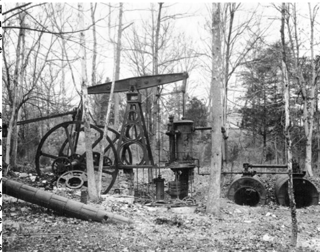
Figure 2: The Vaucluse beam engine in Orange County, Virginia, at the time of its salvage in 1931, showing paired flywheels and two modified Cornish-type boilers.
