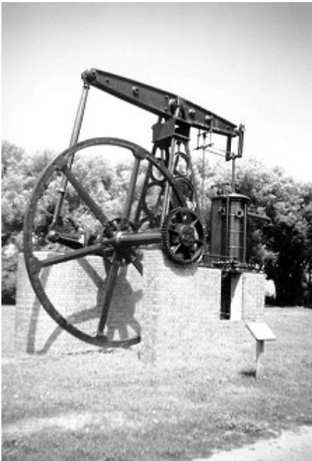
Figure 1: The Vacluse beam engine in Colorado Springs in 1996, showing the slender flywheel and sweep rod, spindle-shaped crank, "indoor" location of the condenser and boiler feed pump, and beam mountings attached to the outside of a beam that lacks a central stiffening rib.
