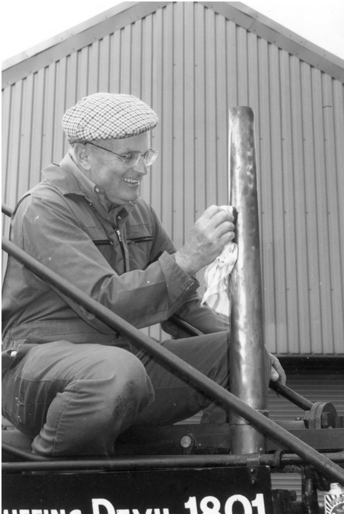
Trevor Thompson, a member from Bristol, shines the copper funnel, which encloses the safety valve on the Camborne road locomotive. Photograph taken by Phil Hosken at the bicentennial celebrations in Merthyr Tydfil.
