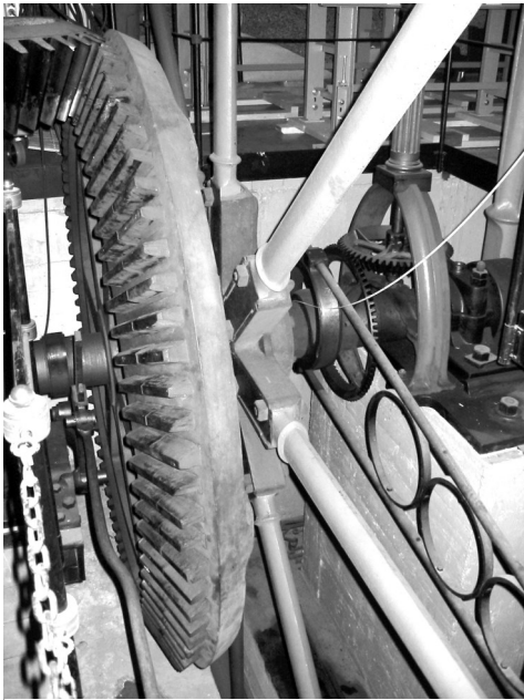
Figure 6: Detail of Watt engine's gearing, cam expansion valve and eccentric rod (2003).
