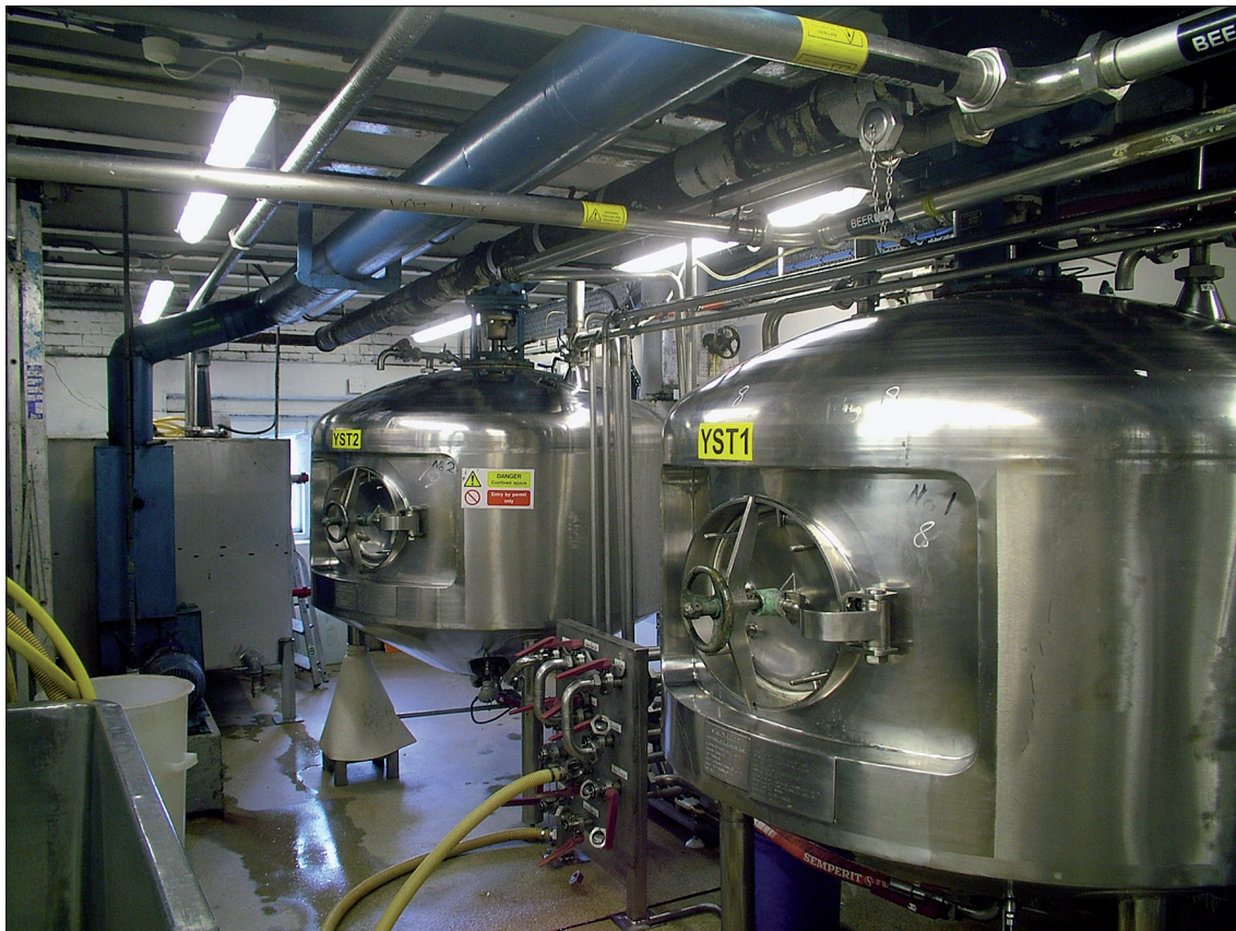
Yeast culture tanks. Yeast is pitched (added) to the cooled wort to ferment the sugars into alcohol and impart flavours. Photo: Steve Barber.
