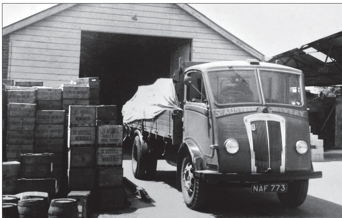
A St Austell Brewery Morris Commercial FV Dray from the late 1940s. The truck was powered by a 4.3-litre six cylinder diesel engine produced under license from Adolph Saurer AG. More commonly on the domestic market it was fitted with a four-cylinder Morris petrol engine delivering a claimed maximum 80 bhp of power.
