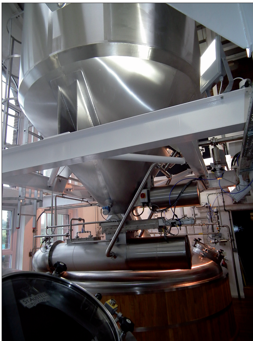
Grist case and Steele's masher. The cracked malt is mixed with hot liquor (water) and fed into a mash tun. Photo: Steve Barber.
