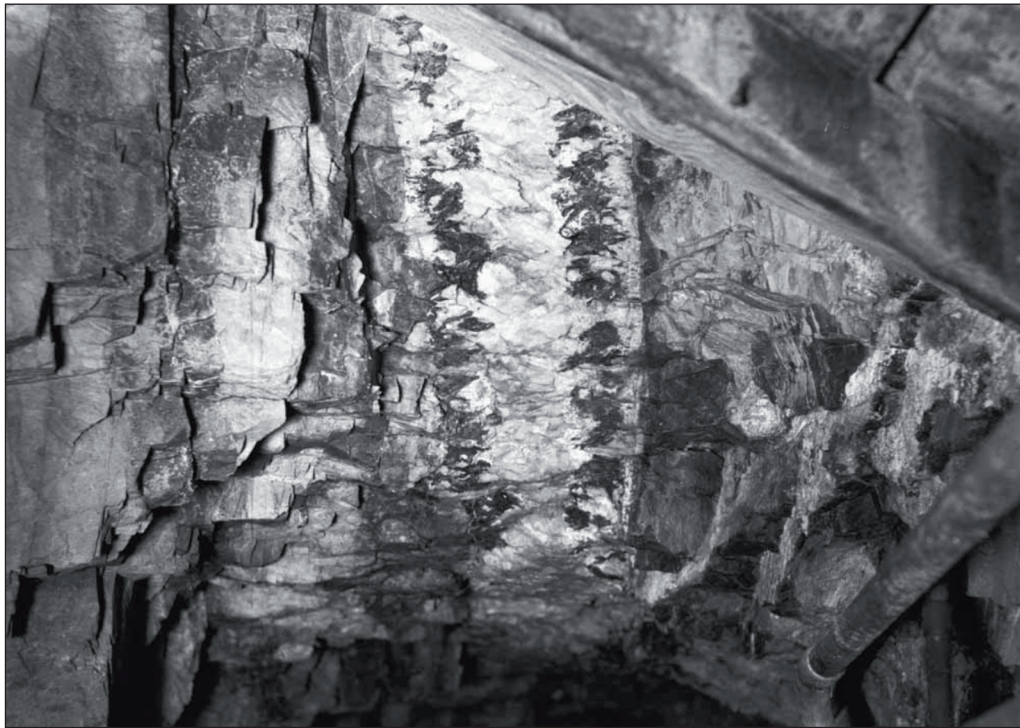
The Wolfram Lode. This exposure, in the back of 5th Level, south of New Shaft shows the lode, about 2 feet wide, of white quartz, with clusters of wolfram crystals along its margins. The killas country rock adjacent to the lode is tourmalinised for a foot or so and, beyond, is white, soft and friable.
