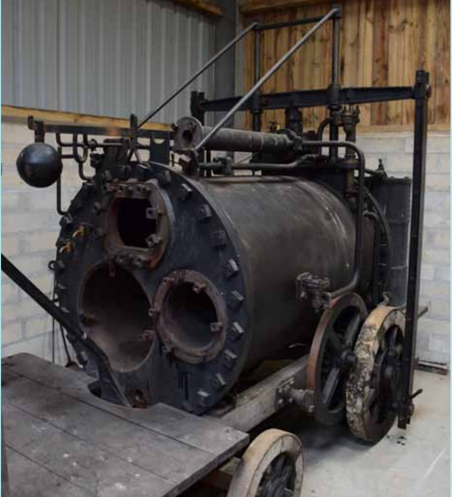
The Puffing Devil stripped down ready for its second ten year boiler test.
