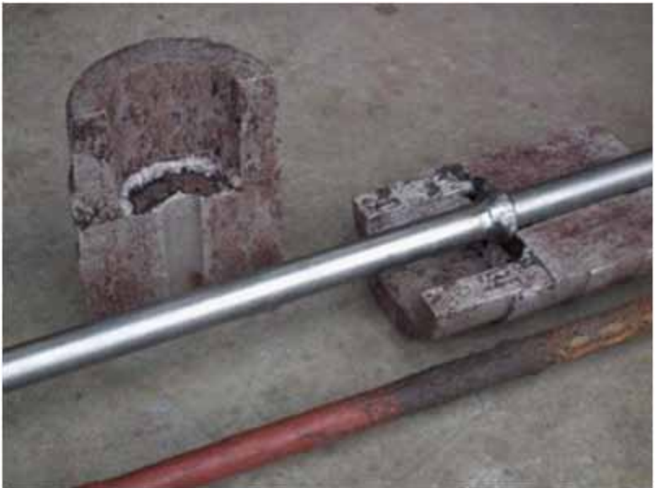
Old and newly manufactured galvanised condenser rod for Levant engine
