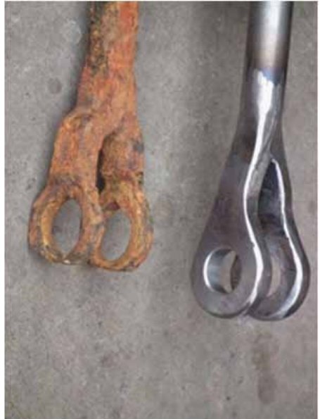
Old and newly manufactured galvanised condenser rod for Levant engine
