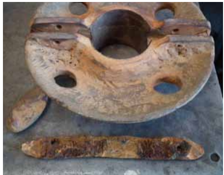
Bronze diaphragm casting and cross peg
