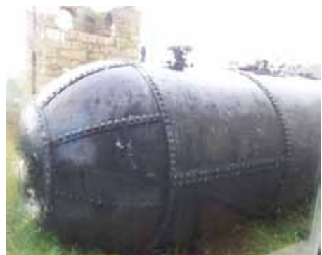
Cornish boiler, King Edward Mine.
